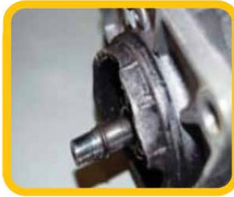
Broken Bracket Incorrectly fitted or vehicle/operator fault, starter engaged while engine is running
