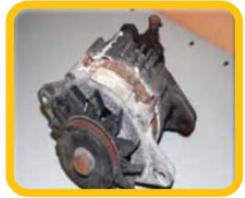
Water Ingress Unit has been immersed in water, vehicle has been driven through flood or deep standing water
