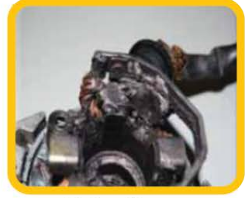
Oil/Diesel Ingress Fuel or oil leak on vehicle dripping onto unit
