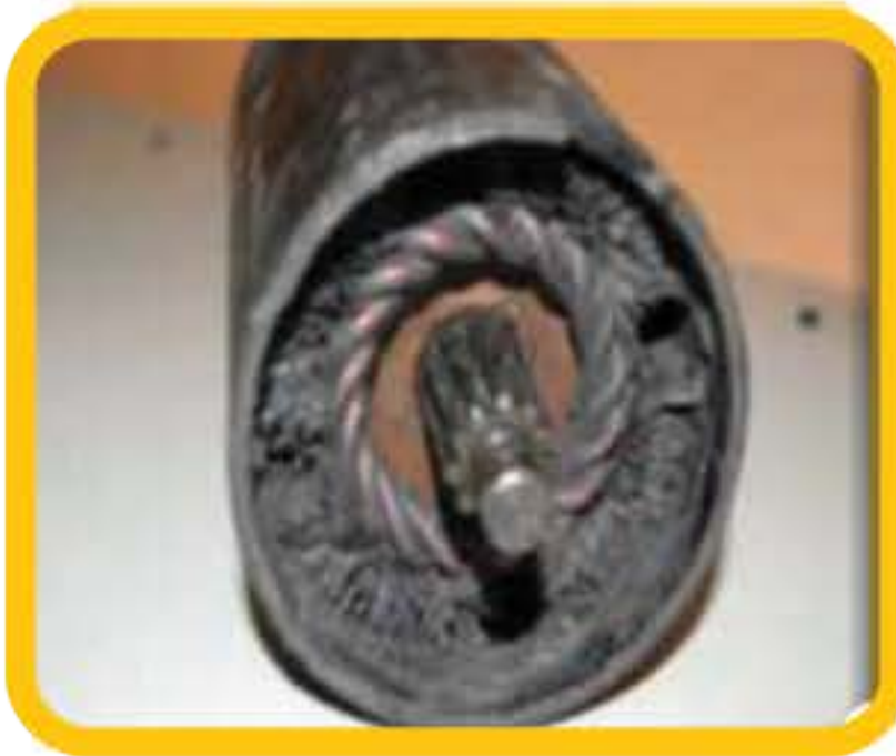
Clutch Dust Build up of clutch dust on gear shaft, solenoid clicks but starter does not engage
