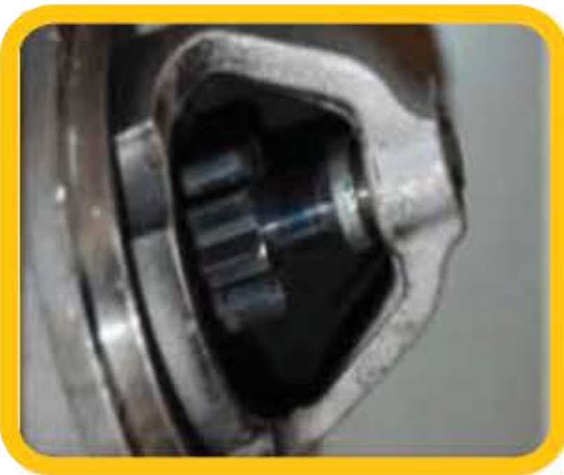
Blue Pinion, Vehicle Fault Starter has been engaged while the engine has been running
